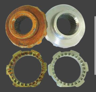
Maximize protection by overlapping Cortec® VpCI® systems: At left, unprotected sintered parts were corroding after 15 hours of ASTM D-1735 testing in a 100% relative humidity chamber at 100.4 °F (38 °C). At right, parts protected in dual system of VpCI®-146 paper inside a VpCI®-126 bag remained corrosion free after 427 hours in the same test conditions.
