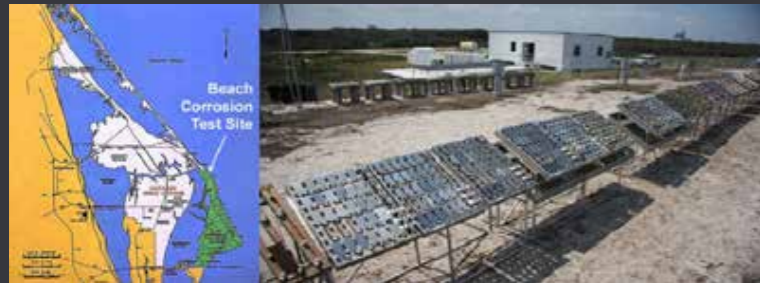
Location of the beachside corrosion test site at Kennedy Space Center, Florida, along the Atlantic Ocean (left) and panels after initial CPC application and exposure to the marine atmosphere at
