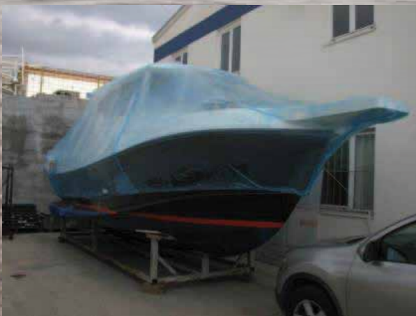
Figure 17. Corrosion protection of yacht on dry berth Protection of electrical circuits and control boxes located on coastal area of Croatia
