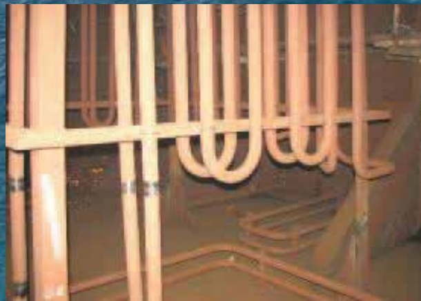
Figure 9. SHIP - ASPHALT CARRIER, 12 asphalt storage tanks /1 tank = 1000 m 3 , VpCI 645 (100 ml/m 3 The use of corrosion inhibitors in the preparation of metal surfaces per tank)
