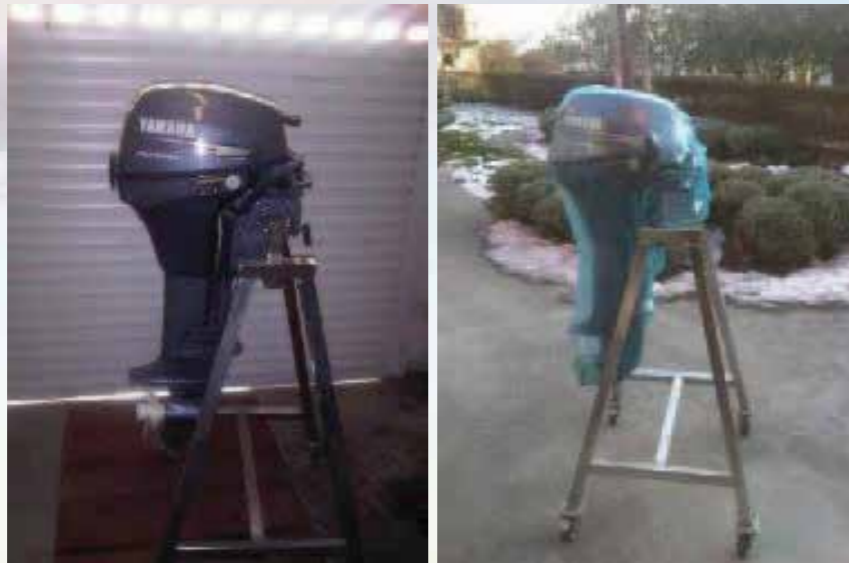
Figure 16. Outboard engine wrapped in VpCI® Film
