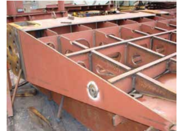
Figure 4. Inside the structure of the rudder
