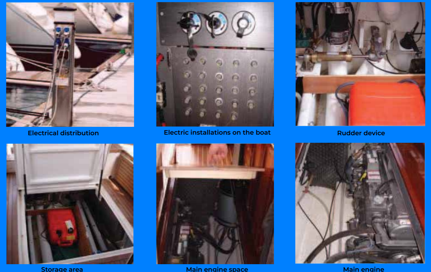
Figure 15. Parts of the boat and nautical equipment suitable for use VpCI® corrosion inhibitors
