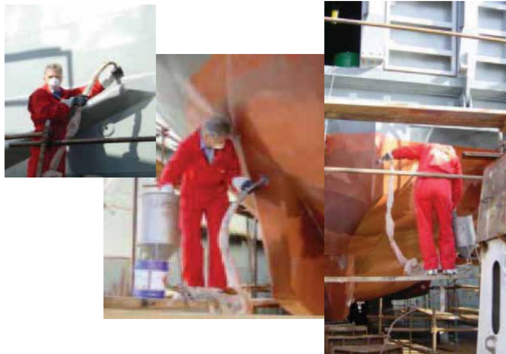
Figure 6. Application of VpCI® inhibitor to keel, rubbing strip and bow of the boat.
