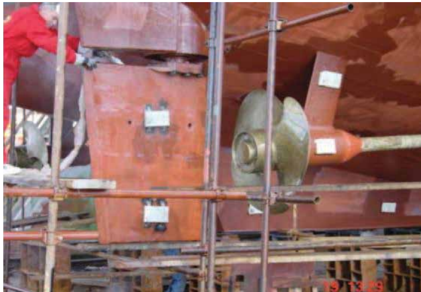
Figure 3. Protection of the rudder blade with VpCI®
