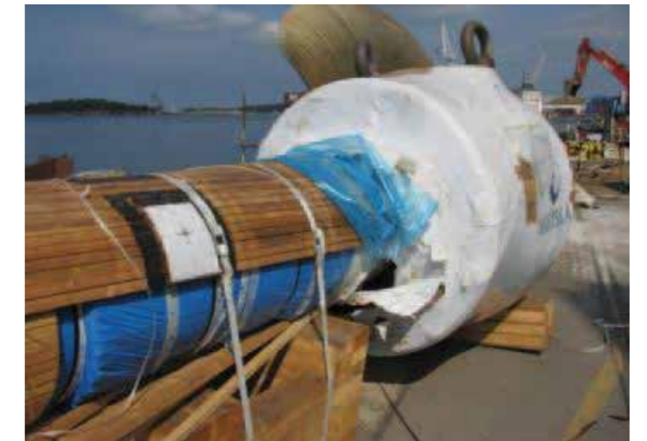
Figure 8.b Protection of equipment with VpCI® 126 film
