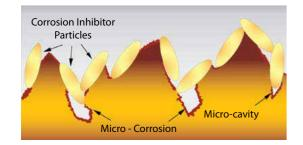
Traditional coatings can not protect the micro-cavities due to the relative large size of corrosion inhibitor particles such as nitrate, aluminum, zinc, and so on. That's where micro-corrosion starts when using traditional coatings.
