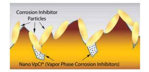
Cortec® Coatings are unique because the Nano VpCI® (Vapor phase Corrosion Inhibitors) penetrates and protects the micro-cavities against micro-corrosion.
