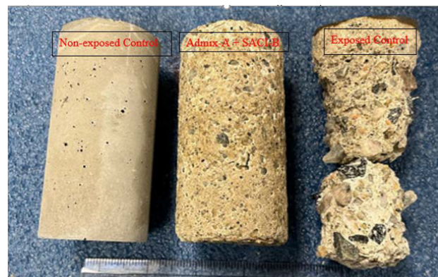
Sulfate attack layer thickness after 400 days exposure to highly acidic solution shows that Admix-A+SACI-B have the lowest sulfate reactions
