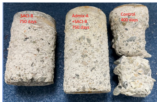
Sulfate attack layer thickness after 750 days exposure to highly acidic solution shows that Admix-A+SACI-B and SACI-B still maintained their strength
