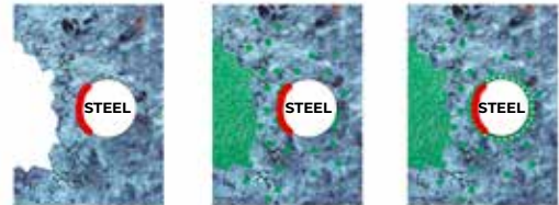
Remove spalled concrete from deteriorating structure. MCI® migrates through concrete without direct application to steel. MCI® protects steel from further corrosion.
